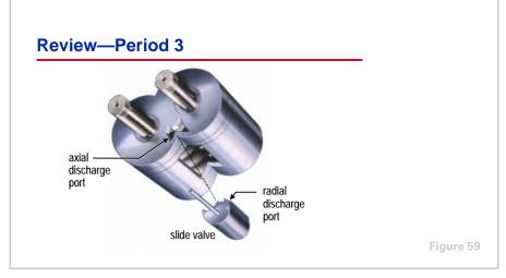
In Period 3, the operation of the modulating slide valve was explained. The slide valve is one method by which a helical-rotary compressor's capacity is controlled.
